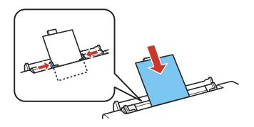
• If loading an envelope, insert it short edge first with the flap facing down, in the center of the rear paper feed slot. Slide the edge guides against the envelope, but not too tightly.
